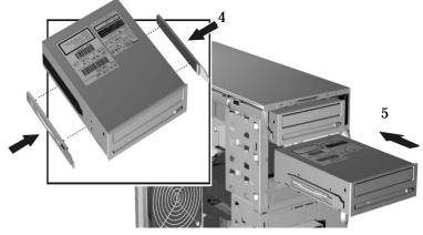
5. Connect the power and data cables to the installed device. The connectors are shaped to go in one way only. If you are not sure which connector to use, refer to "Mass Storage And Optical Device Overview" on page 125.
